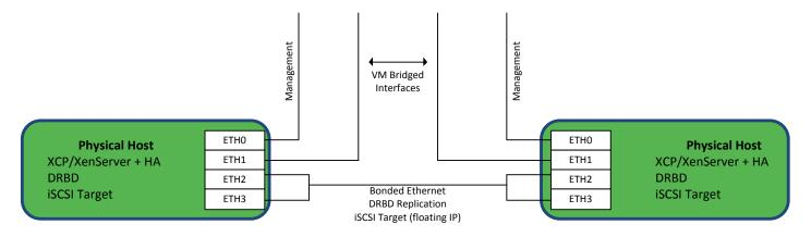
In this example, the DRBD and iSCSI interface is provided via direct attachment (no Ethernet switches) on a bonded Ethernet link. This approach greatly eliminates the possibility of a split brain scenario since there are no networking devices interconnecting the hosts in any way. Additionally, utilizing a bonded Ethernet link further eliminates the possibility of communication interruption between the hosts.
