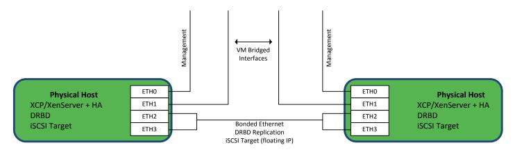
In this example, the DRBD and iSCSI interface is provided via direct attachment (no Ethernet switches) on a bonded Ethernet link. This approach greatly eliminates the possibility of a split brain scenario since there are no networking devices interconnecting the hosts in any way. Additionally, utilizing a bonded Ethernet link further eliminates the possibility of communication interruption between the hosts.
